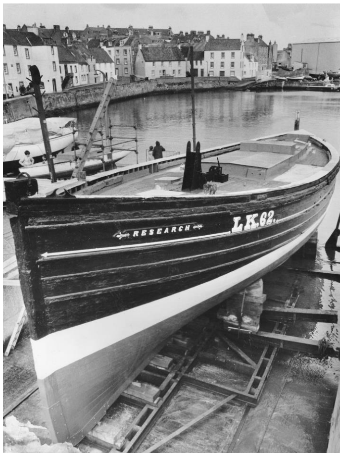
The 78ft, Research LK 62, a 1901 Zulu type herring drifter after having a new keel fitted at James N Millers, owned by the Scottish fisheries Museum
